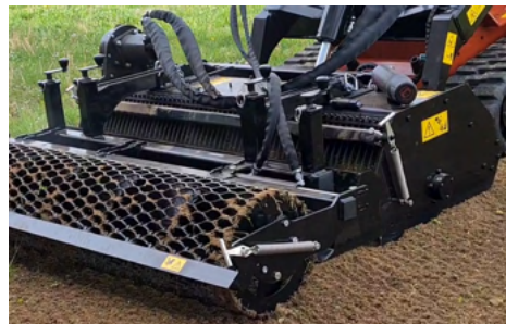
Option : Roller side adjustment device by cylinder
