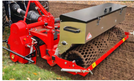
Option : Stainless Steel Gravity Grass Seeder (SG)
