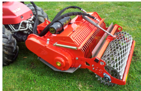
Option : Working depth setting by hydraulic jack
