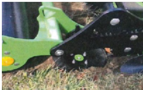
Option : edge trimming with sharpened disc
