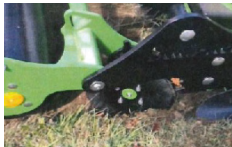
Option : edge trimming with sharpened disc
