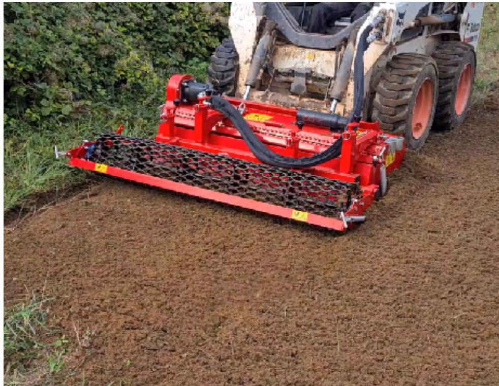
- Gravity Grass Seeder : SG 130 for RDH 52 and SG 145 for RDH 60 - Spiral roller
