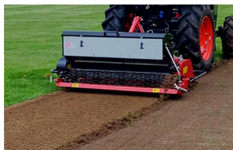
Option : Stainless Steel Gravity Grass Seeder (SG)
