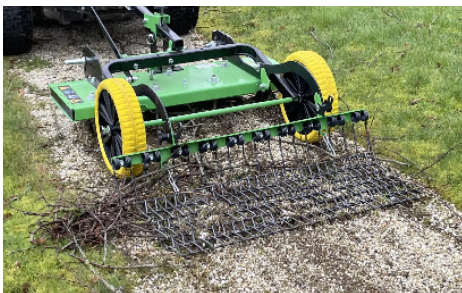
Rake, harrow and grid for clod crumbling
