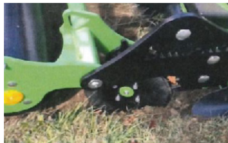
Option : edge trimming with sharpened disc
