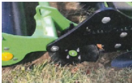
Option : edge trimming with sharpened disc
