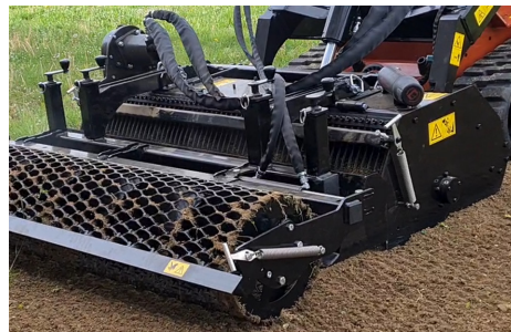
Option : Roller side adjustment device by cylinder
