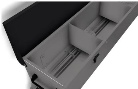
Mixer for decompacting seeds in the seedbox
