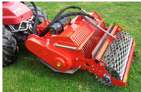
Option : Working depth setting by hydraulic jack
