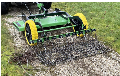
Rake, harrow and grid for clod crumbling
