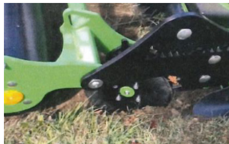
Option : edge trimming with sharpened disc
