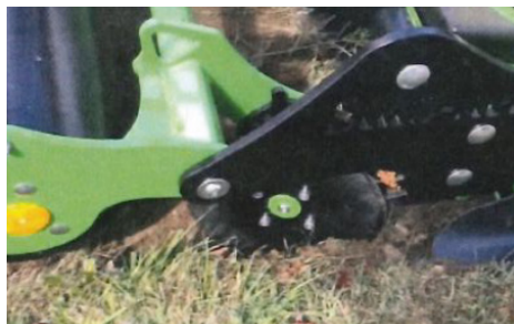
Option : edge trimming with sharpened disc
