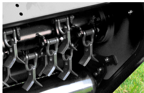
Y-shaped mounting of knives on shackles
