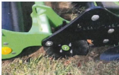
Option : edge trimming with sharpened disc
