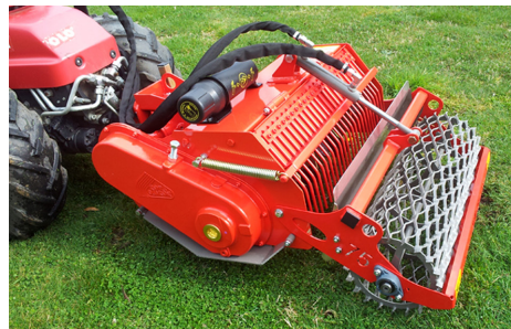
Option : Working depth setting by hydraulic jack
