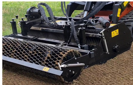
Option : Roller side adjustment device by cylinder
