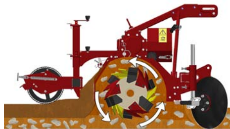
Soil preparation principle
