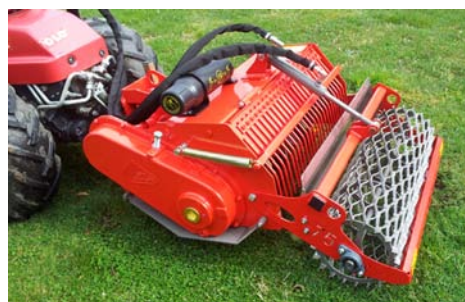
Option : Working depth setting by hydraulic jack
